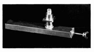
Tunable waveguide diode mount with TWT or BWO N connector.
